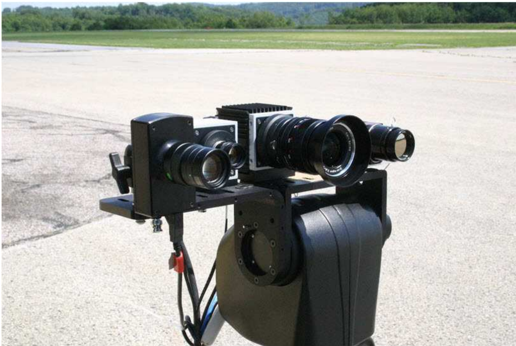
Figure 7: Directed Perception D-100 pan tilt unit was used along with a geo-pointing module to automatically keep the approaching aircraft in the field of view of the mounted cameras. The pan tilt unit tracked the location of the approaching aircraft using the GPS stream over a radio modem from the aircraft.
