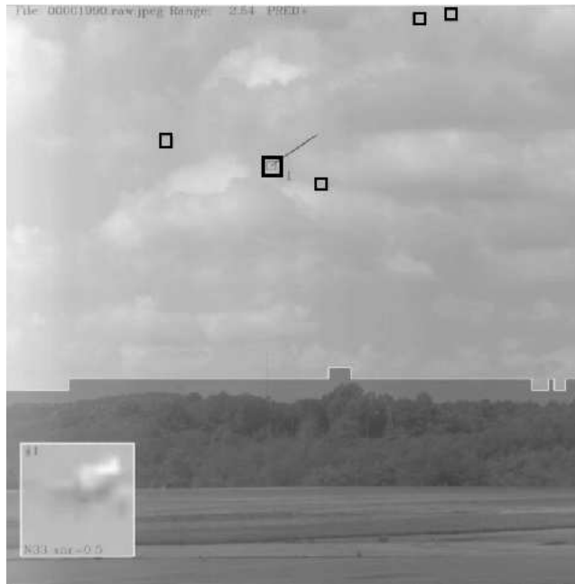
Figure 6: Stage 3 output on example image. The detected track history of the actual aircraft in the image has been overlaid as a black trail on the image. The actual aircraft position is represented by the bold black box and the detected and tracked position by the smaller black box which is shown positioned on the groundtruth location. The other black boxes represent detected dead pixels and detected dust particles on the camera lens. There are no false positives remaining in Stage 3 in contrast to Stages 1 and 2. See Fig.3 and Fig.5. The inset image on the bottom left of the figure shows the aircraft zoomed in on the example image as detected by the algorithm.
