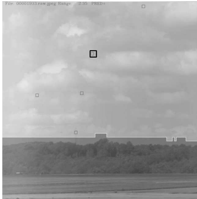
Figure 5: Stage 2b output on example image. The points of interest detected by the morphological filter in Stage 1 are assigned probabilities by a trained Support Vector Machine (SVM) of being true positives. Only those detections which exceed a minimum value are kept. This step eliminates a large percentage of the false positives. As compared to Fig.3 the above image contains only a few false positives. The true location of the aircraft in the image is represented by the bold black box and the remaining points of interest after SVM based false positive elimination are shown by black boxes. In spite of the elimination of a large percentage of the false positives, the true positive (inside the bold black box) is correctly preserved.
