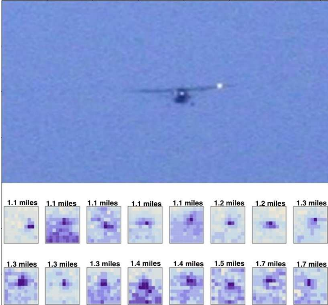
Figure 1: Selection of 11 \times 11 subwindows showing the image of the Piper Archer II which was used as the approaching aircraft for collecting imagery, at a range of 1.5 miles. The camera and lens used had 0.41 milliradian/pixel resolution and a field of view of 30^\circ(\text{H}) \times 21^\circ(\text{V}) .
